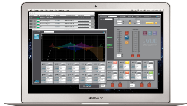
Fig. 26 - SystemVUE software interface (unit control, EQ shown)
