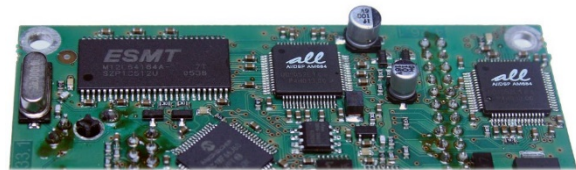
Fig. 23 - Integrated DSP for processing and system management functions in all VUE Drive Systems Engines variants
