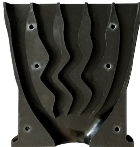
Fig. 13 - High-frequency waveguide assemblies incorporate path-length optimized internal channels to create a time-coherent pressure wave across the entire exit aperture.
