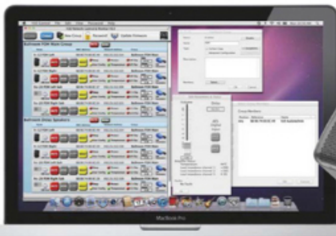
VUE Control Software offers remote control and monitoring of DSP and amplifier parameters in self-powered I Class speakers.
